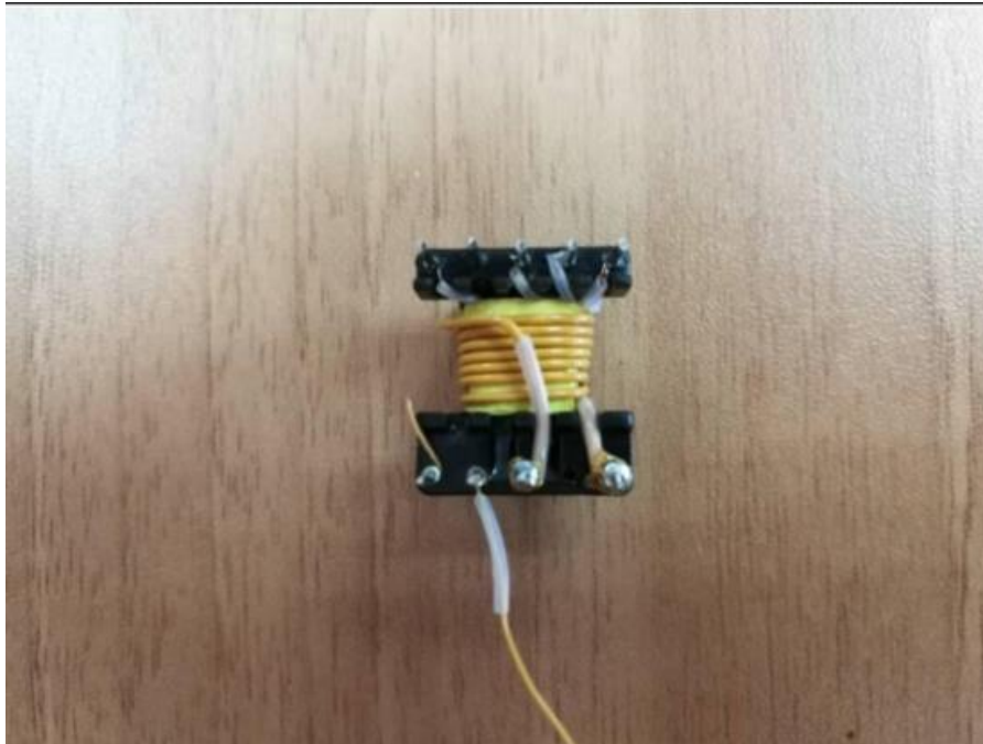
Triple-insulated secondary winding
