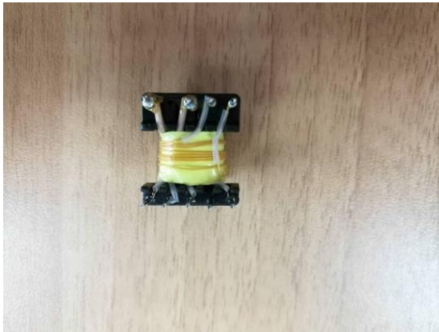
Triple-insulated secondary winding
