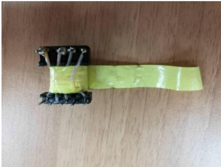
Triple-insulated secondary winding
