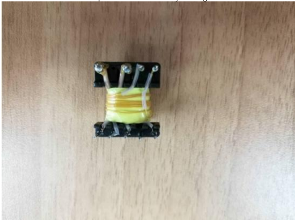
Triple-insulated secondary winding
