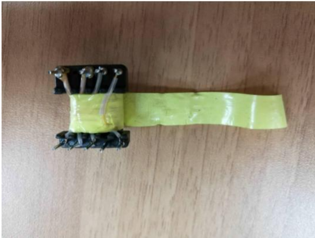
Triple-insulated secondary winding
